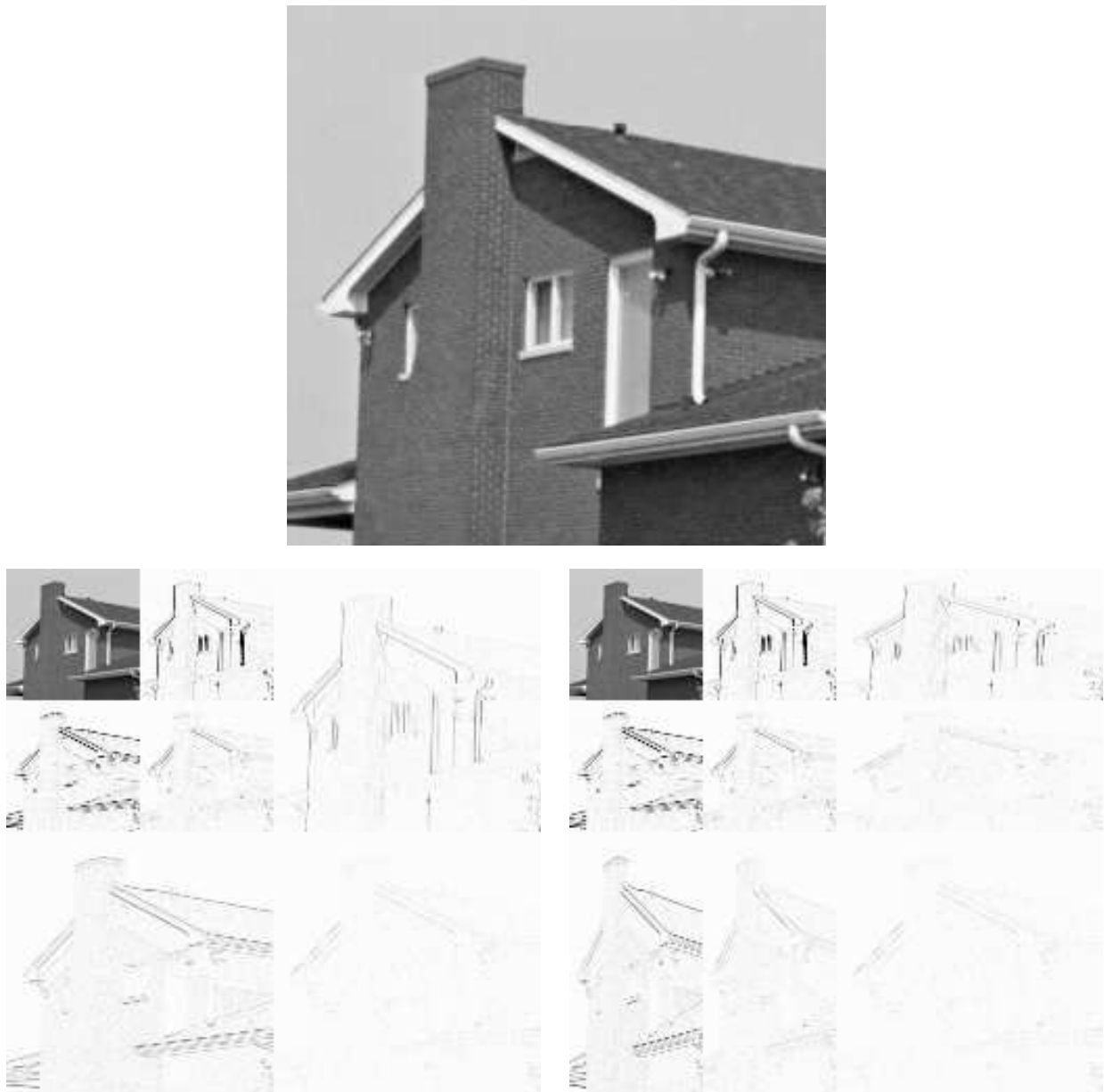
Figure 8.3: Image and its wavelet transform
