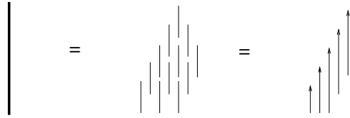
FIGURE 3.4. Givens factorization of a unitary transformation of the left branch of a Givens product representation. Note that this figure is precisely transposed to Figure 2.3.
