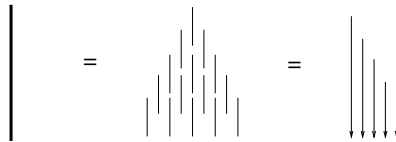
FIGURE 3.3. Givens factorization of a unitary transformation of the right branch of a Givens product representation. Note that each unitary matrix allows such a factorization.
