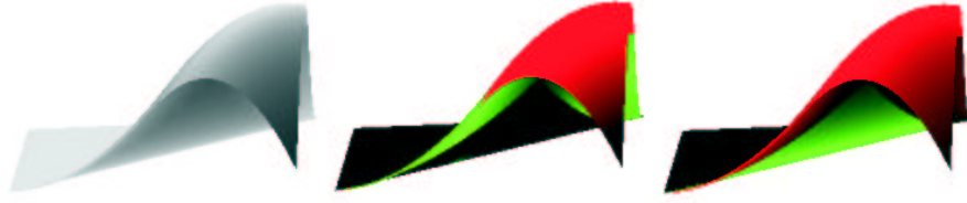
Figure 6: Left: A smooth PS-surface. Middle: Gaussian curvature plot of the PS-surface. Right: Mean curvature plot of the PS-surface.
