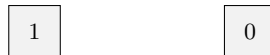
Fig. 16. The two most simple BDDs, (left) the 1-terminal represents the constant function true , and (right) the 0-terminal represents the constant function false .
