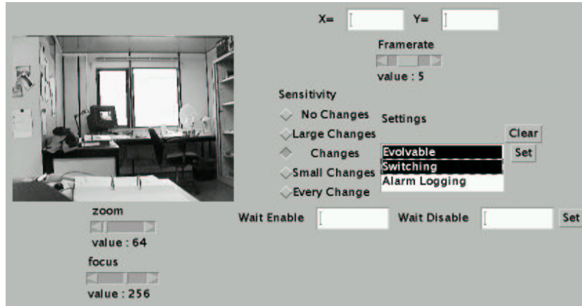
Figure 3.3: GUI of the camera (left side) and the motion detector (right side)
